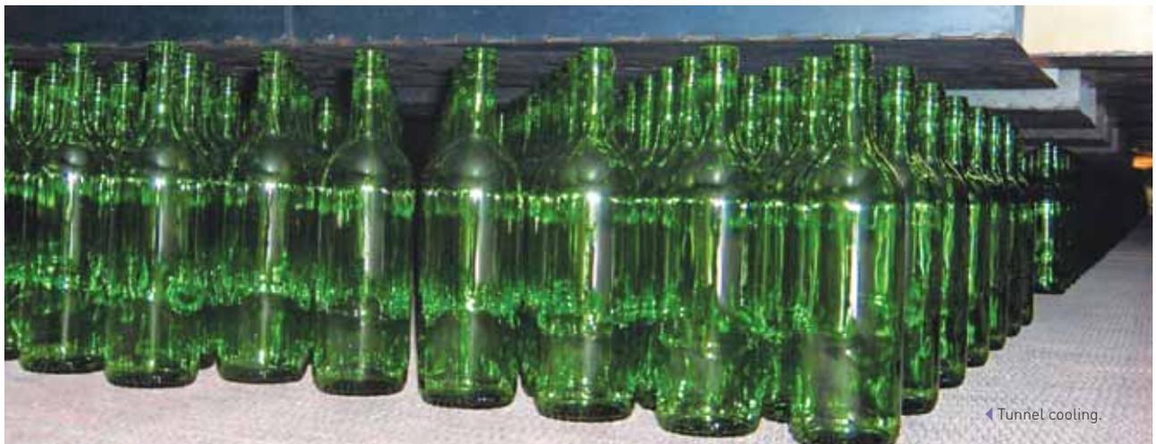
to bring the glass to a state of temperature equilibrium (molecules in similar state of expansion through Viscous flow) and prevent variation in cooling rates as the glass passes below the strain point. If the following for a glass container is assumed:
